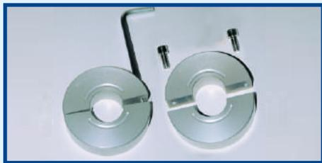
**3** Set both of the Ring halves onto the prepared section of the pipe.
