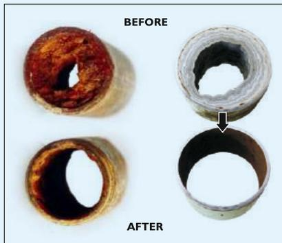
This picture shows one of many practical examples of before and after installation of a WELLAN® 2000 Ring. The pipe on the right shows the result after just 8 weeks of use. The lime crystals are disintegrated by the natural oscillations of the WELLAN® 2000 Ring and the dissolved lime is carried away with the flowing water.
